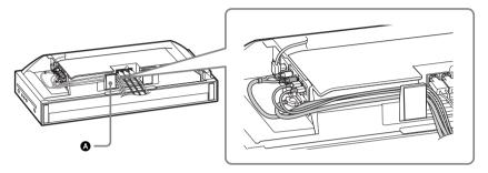
3 Thread the AC power cord (mains lead) through the gap on the bottom of the unit by securing it behind the tabs, and then draw it around the rear support (19).
